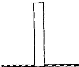
This perforated plate is laid on the bottom of a dish or crucible made of platinum, porcelain, or any other suitable material. The upper portion of the tube is connected with an aspirator, and there must be a small space left between the under surface of the plate and the bottom of the vessel, to allow the filtered liquid to pass through the filtering medium. The liquid which passes into the space under the plate, is removed through the tube by the action of the aspirator.
