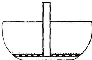
The filtering medium may be a piece of filter paper, or it may be deposited in the form of paper pulp or asbestos pulp, as already mentioned. If a paper filter is used, there should be a hole in it, to let the tube go through. The perforations in the plate should begin at a certain distance from the tube, so that every portion of the perforated surface may be covered with paper.
